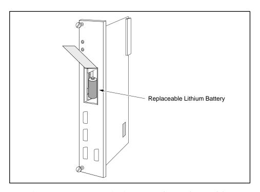
Figure 3-9 Battery Location in -1105 and -1106 CPU Modules
