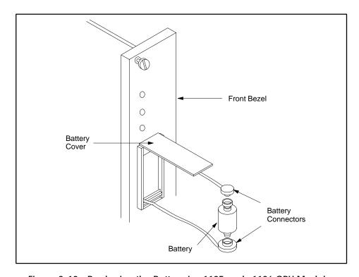
Figure 3-10 Replacing the Battery in -1105 and -1106 CPU Modules
