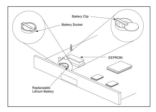
Figure 3-11 Battery Location on 545/555 CPU Modules
