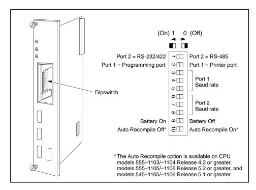
Figure 3-12 545/555 CPU Dipswitch Location
